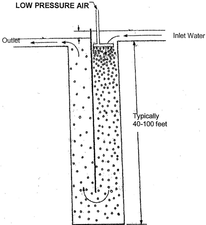
Figure 4.8 – Schematic of Compressed Air U-Tube Contactor
