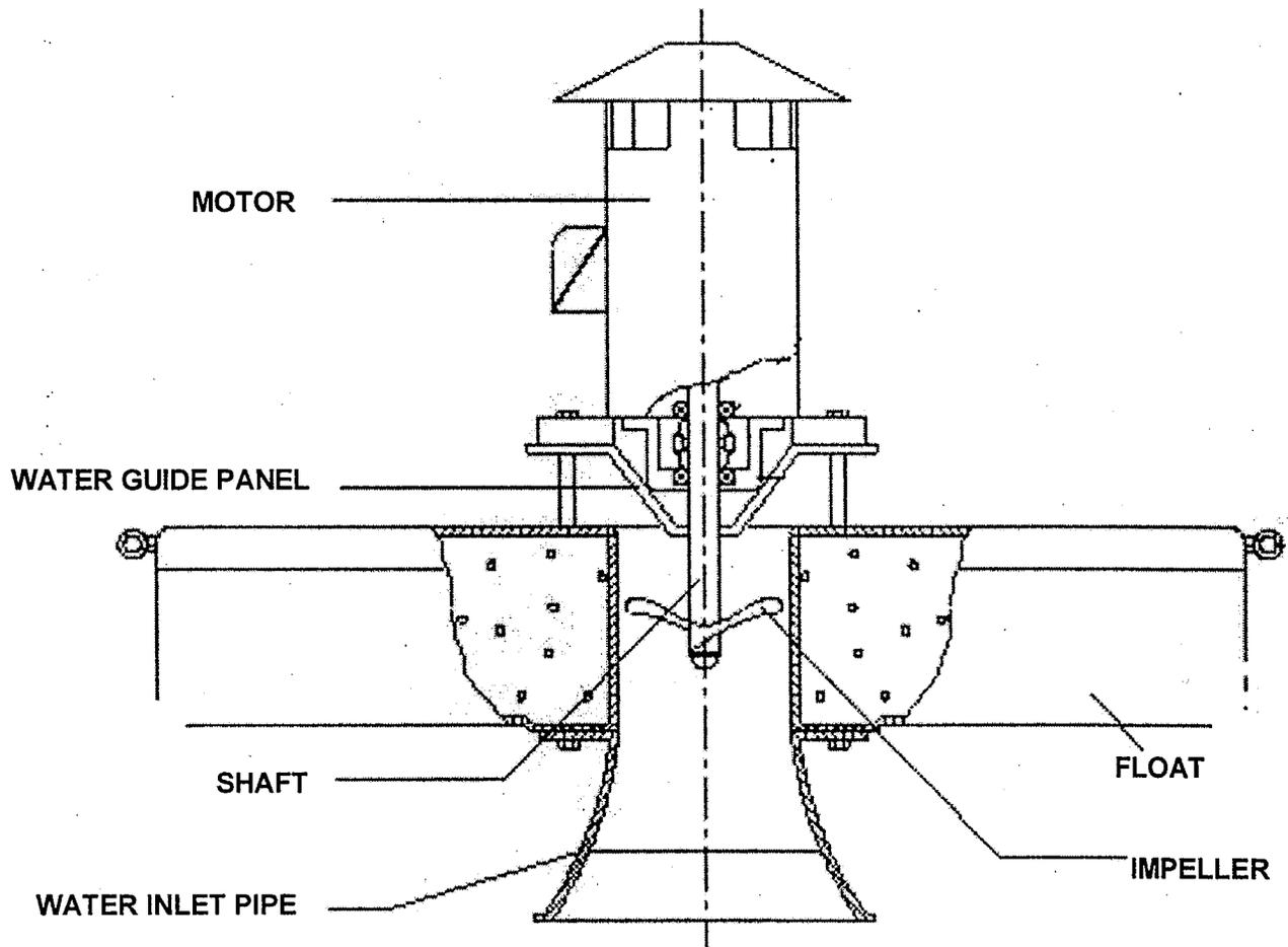
Figure 4.7 – Mechanical Surface Aerator
