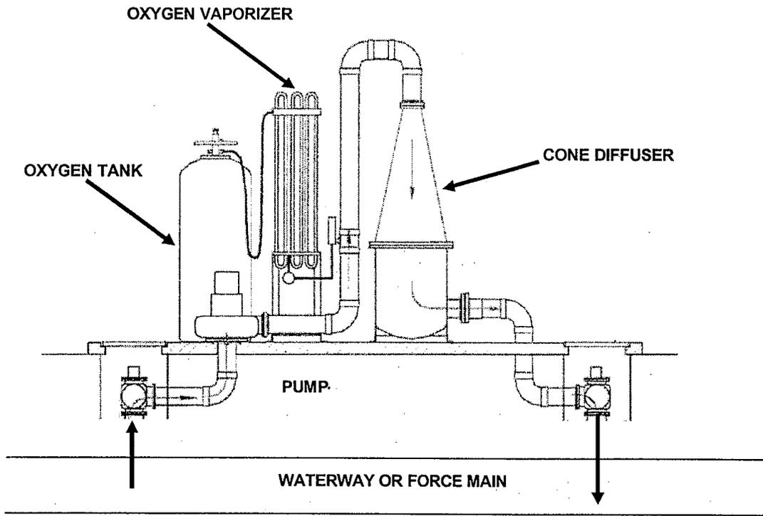
Figure 4.9 – Schematic of Pressurized HPO Contactor
