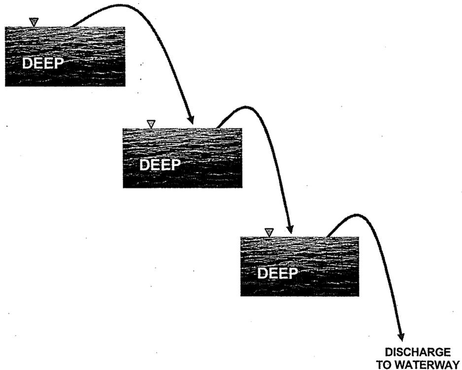
**Figure 4.6 – Schematic of 3-Step Weir Supplemental Aeration System**
