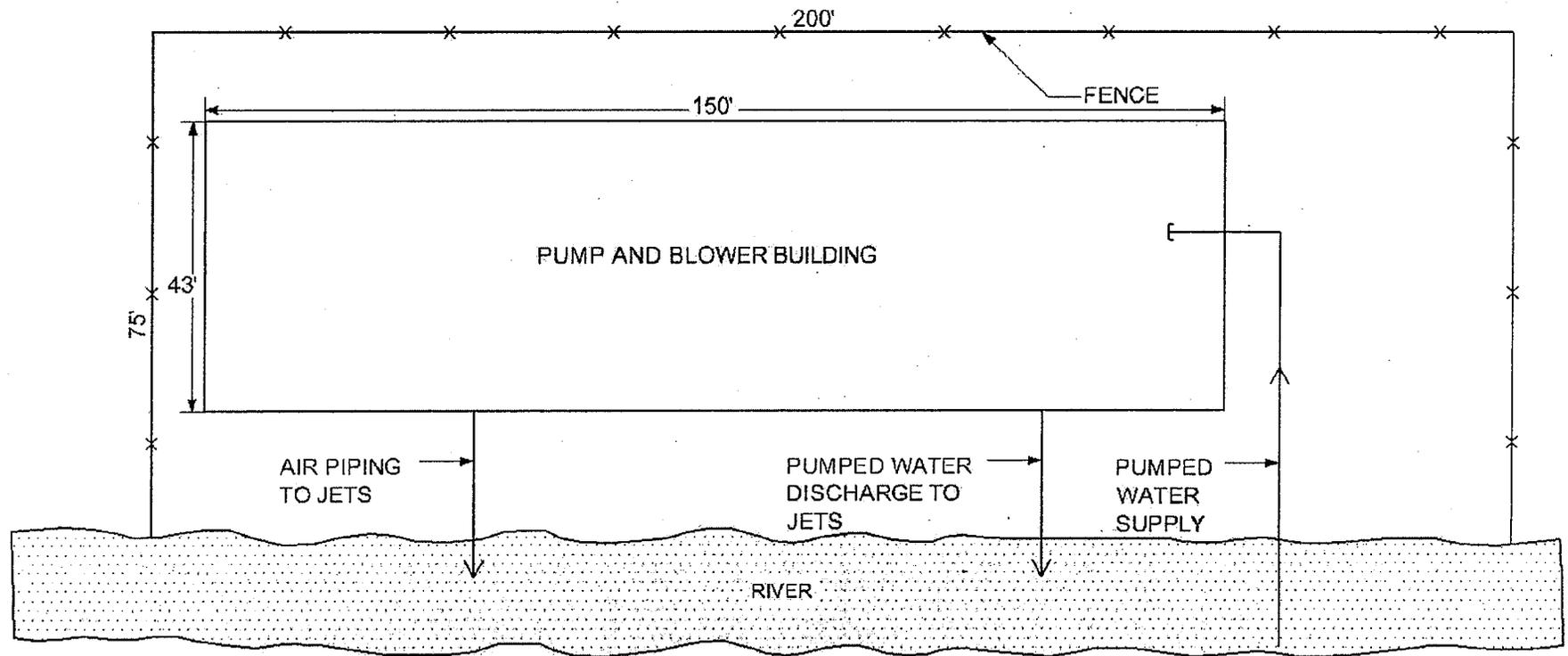
Figure 4.12 – 80 g/s (Oxygen) Jet Aeration Station Conceptual Layout
